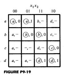
9-22 Find a circuit that has no static hazards and implements the Boolean function:
